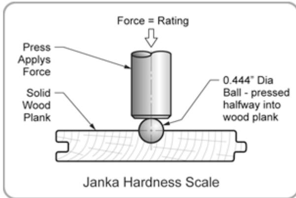
The [Janka Hardness Scale](#) measures the hardness of wood and is typically referred to in comparing the hardness of wood flooring types. Created in 1922, the first Janka rating results were given in units of pressure (Pa). It wasn't until the test was standardized in 1927 that the results were given in units of force (F).
